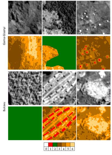
**Figure 2.** Sample training images from Goma-Gisenyi (first two rows) and Bukavu (last two rows) illustrating examples of panchromatic images, and the diversity in the layout and appearance of classes. The legend is 1—building, 2—high vegetation, (3–6) mixed bare land and low vegetation. 0 represents the unclassified pixels.
